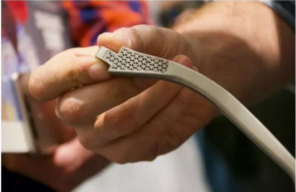
A 3D-printed brake lever demonstrating that a lattice infill can be printed using ADAM without worrying about powder escape cavities. (Image courtesy of the author.)
